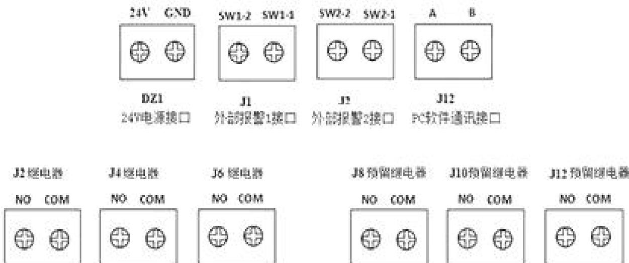
USC4940 吸气式感烟火灾探测器端子布局图 (6-1-1)
